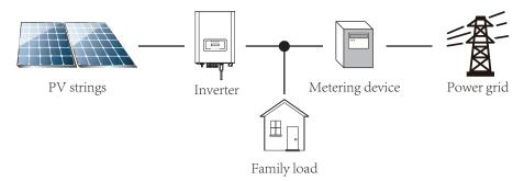
Application of inverter in photovoltaic power system
