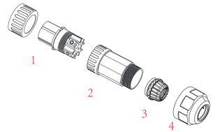
1. Matching socket 2. Sleeve 3. Sealing core 4. Sealing nut Pic 5.7 AC connector structure
