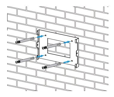
Pic4.5 Inverter hanging plate installation
