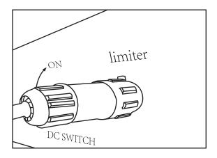
Pic7.7 Connect terminal to inverter
