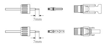
Pic 5.3 Disassemble the connector cap nut
