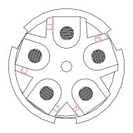
Pic 5.9 AC Connector Hole Pattern
