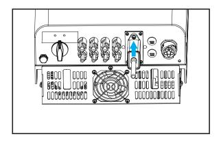
Pic 5.13 Wifi Plug installation diagram
